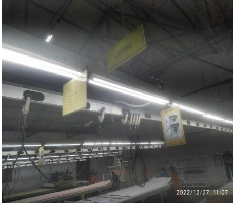
Combustible material found hanged near Electrical sources
