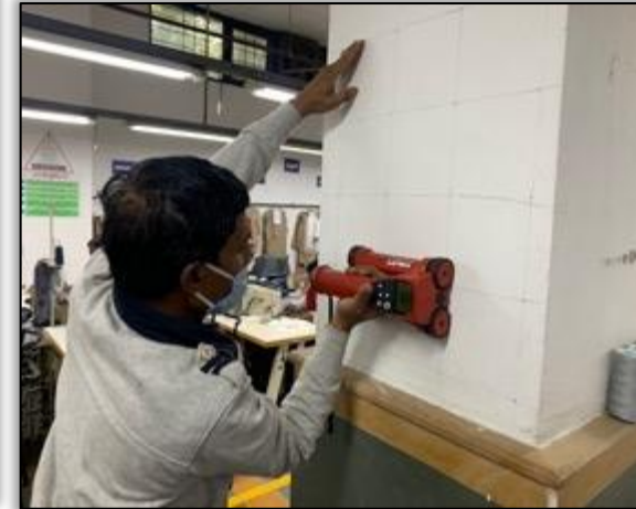
Structural Safety: Ferro-Scanning Test
