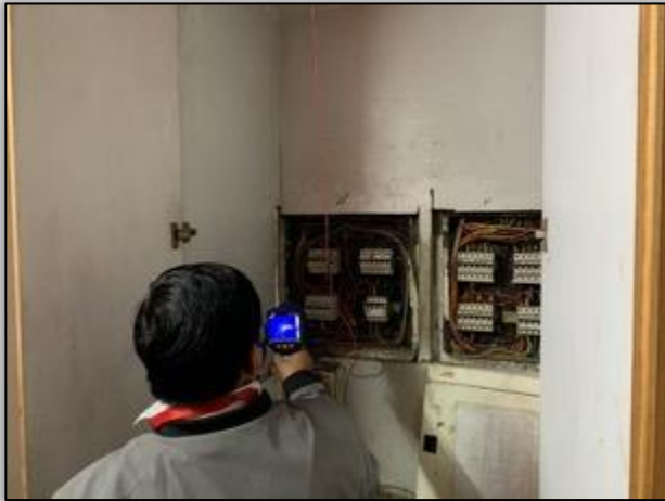
Electrical Safety: Thermo-graphic Test
