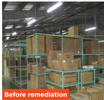
Before remediation In-process storage in production area without fire-rated separation
