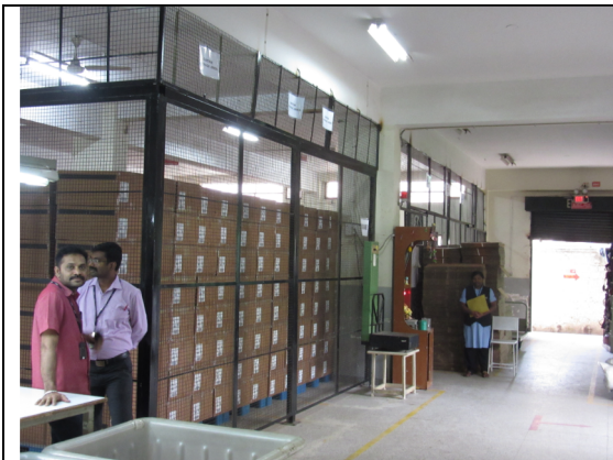
Figure 11 Dedicated storage area separated by open wire enclosure (eg. above)
