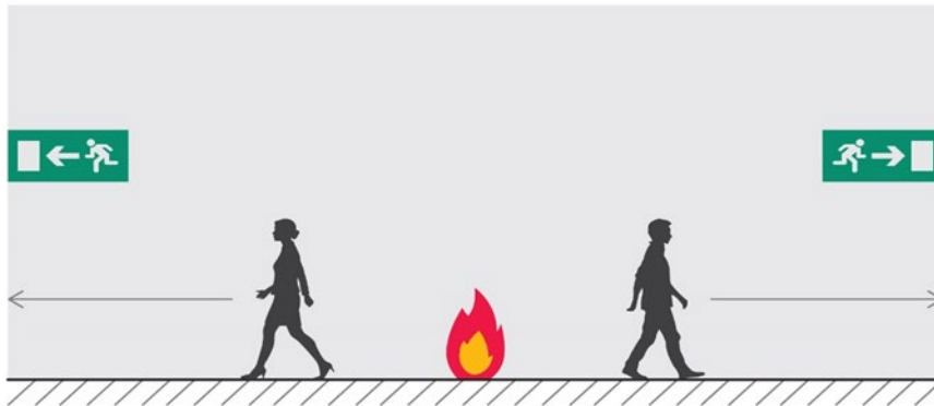
Figure 4 Alternative directions of escape
