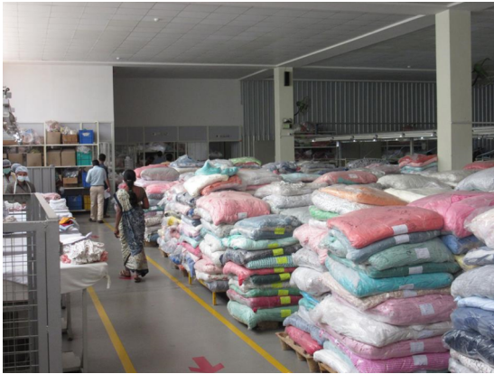
Figure 9 Excessive ‘in-process’ storage stacked on Sewing floor (eg. above)
