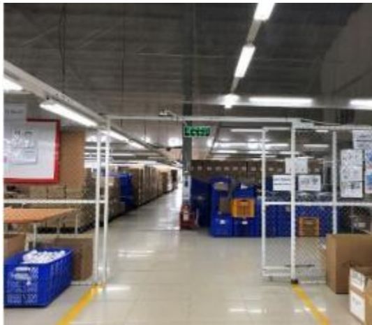
Figure 11 Dedicated storage area separated by open wire enclosure (e.g. above)
